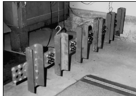
Figure 3b. One of six long-beam assemblies hanging from springs during step-relaxation tests. The short beam series was similar except three weldments were connected back-to-back directly to another three.
